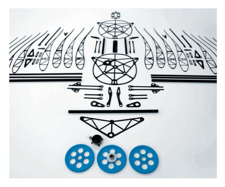
the torso to the wing tips; this movement is conveyed by a trapezoidal joint. At the same time, the wings twist upward during the up-stoke, whereby the correct angle of inclination is crucial. The extent and timing of the twist are controlled by a servomotor. The arm wing thus generates lift, and the hand wing propulsion. This active articulated torsional drive is a feature unique to SmartBird that combines the two movements into a single function.
