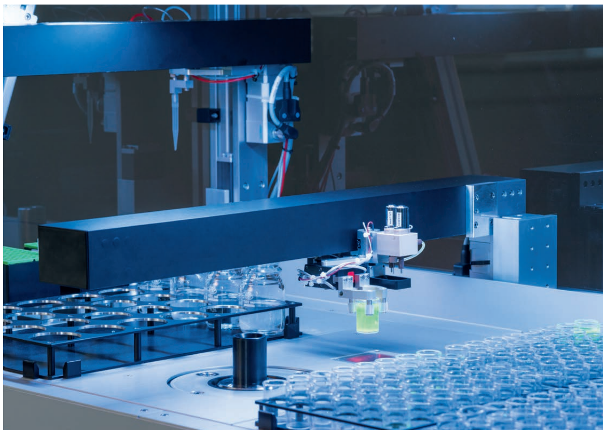
Precise pipetting processes: thanks to compact handling gantries with electric axes from Festo.
