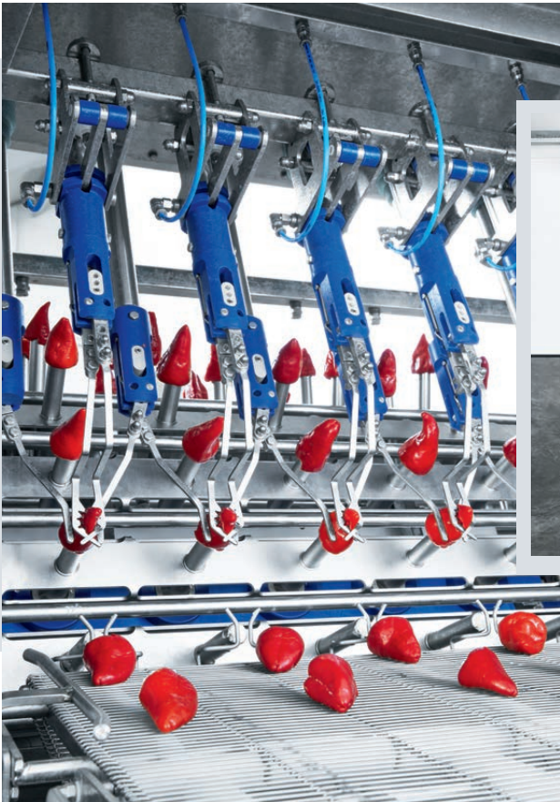
Everything under control: the grippers developed by Karb Maschinenbau use Festo cartridge cylinders EGZ.
