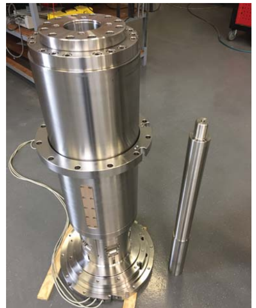
Figure 2: Data regarding the Mechanical Fail safe solution: Type: EMMA 02, Status: Prototype, Force: 50 kN, Stroke: 300 mm, Tension: 400 V
