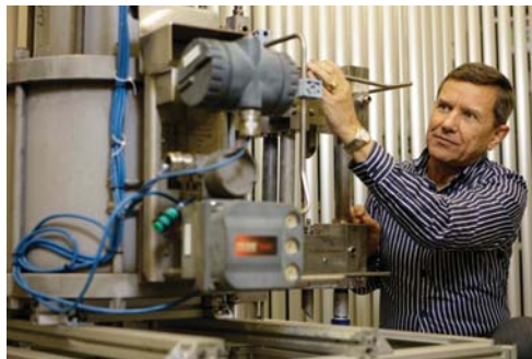
Figure 1: The challenges with pneumatic actuators are legion, for example the complexity, increasing leakages during life cycle, low reaction time in emergency cases, less accuracy in control and hysteresis.
