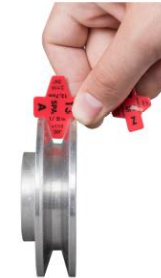
Figure 11. Determining the belt type using the V-belt and pulley gauge.
