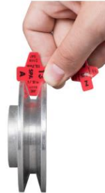
Figure 11. Determining the belt type using the V-belt and pulley gauge.
