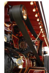
Figure 4. Flat belt in an industrial engine.
