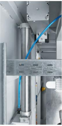
**Landing on the "air cushion":** Two flange-mounted air chambers ensure that the partition closes quickly yet gently.
